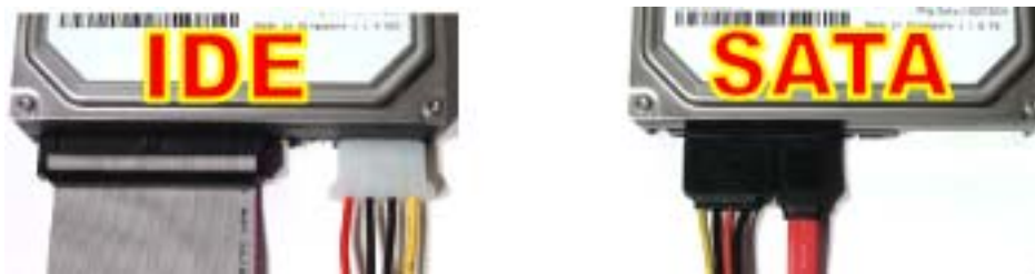
Figure 3: Comparing the interfaces of IDE and SATA hard drives
