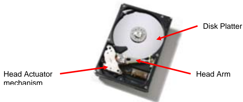
Figure 2: A common 3.5-inch hard drive, with cover removed
