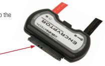
b. Connect the SATA data cable from Encryptor to the corresponding port on the dock.
